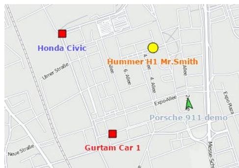
Besides, the colors of these icons (arrow, square, circle) can be different and depend on the value of sensor. This functionality is adjusted on the [Advanced](#) tab of unit properties. In other words, the shape of the icon is defined by the state (standing still — square, moving — arrow), and the color depends on the sensor value (intervals and colors are adjusted in [sensor properties](#)).
