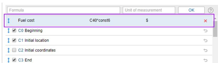
To edit the name, formula, or units of measurement for the created column, click in the desired field with the left mouse button and make the required changes. Click anywhere in the dialog to confirm the changes.
